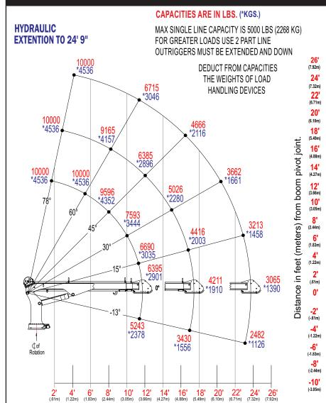
Radius in feet (meters) from centerline of rotation to load.
