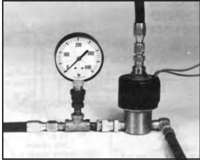
Before 378965 Screen Adapter at "In" Port of Solenoid Valve.
